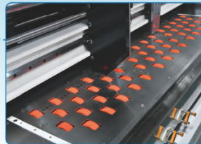
伺服免压前缘吸风送纸。 Servo pressure-free leading edge paper feeding system.
